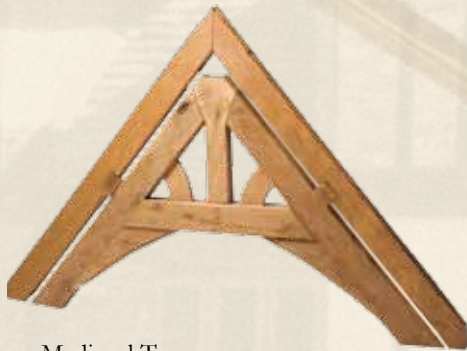
Medieval Truss (with rafters) - these are similar to the King Post style but with the tie beam raised up and knee braces forming an arch
