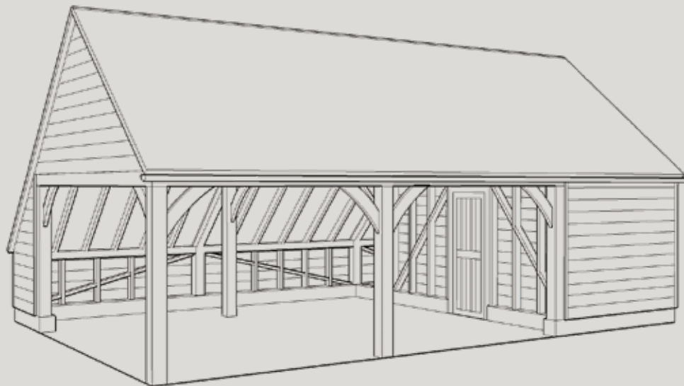
Three bay garage with catslide rear roof, two open bays and one closed
